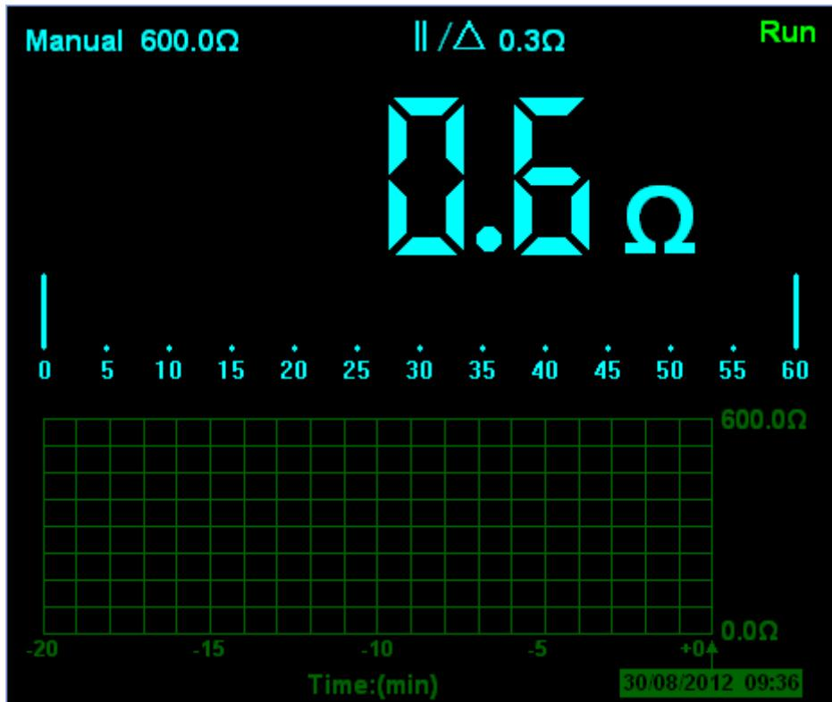
Figure 2-21 Relative Measurement
