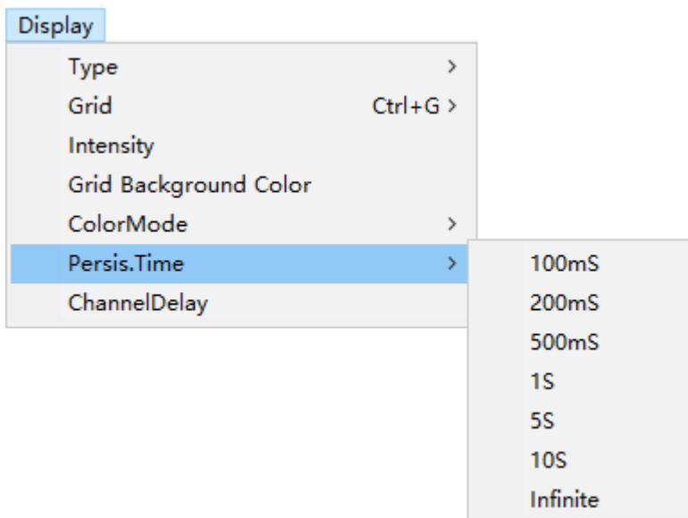
With persistence, the oscilloscope updates the display with new acquisitions, but does not immediately erase the results of previous acquisitions. All previous acquisitions are displayed with reduced intensity. New acquisitions are shown
