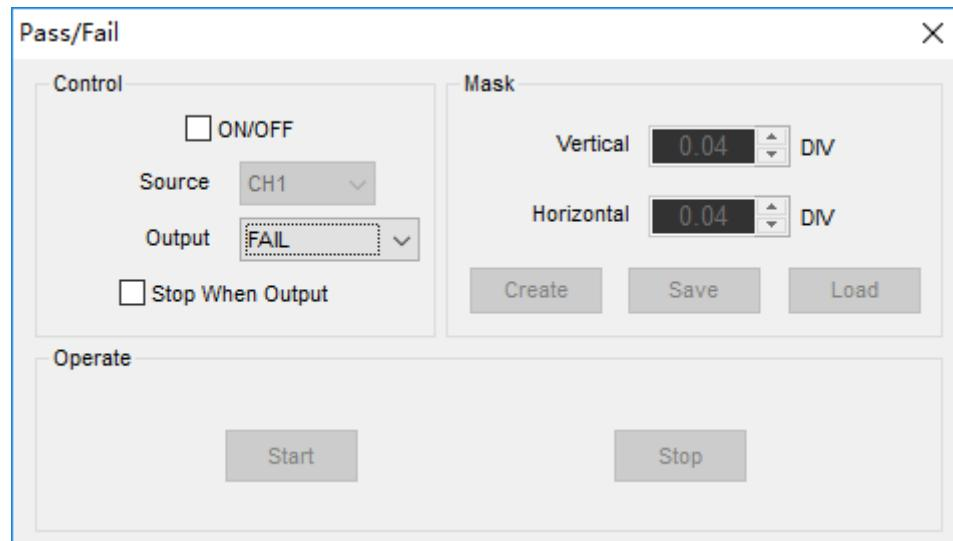
The **Pass/Fail** function monitors changes of signals and outputs pass or fail signals by comparing the input signal with the pre-created mask.
