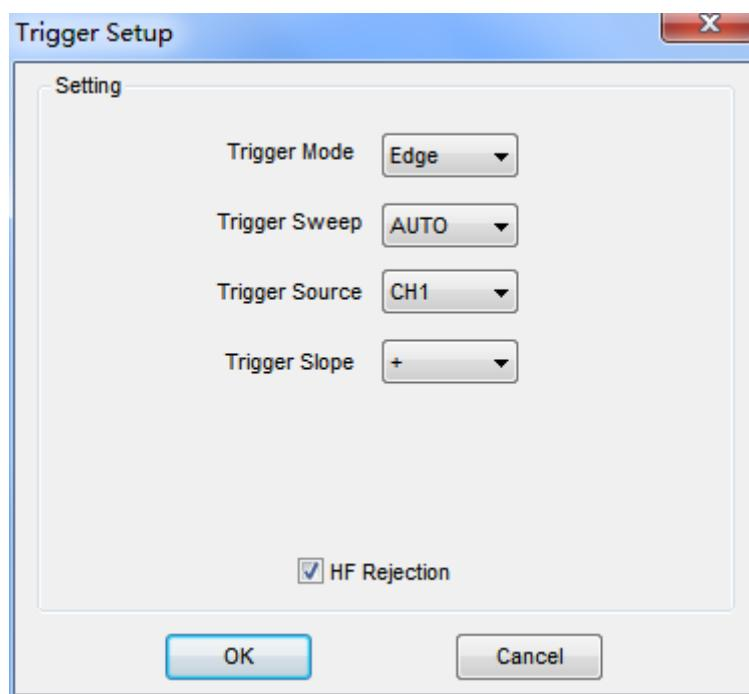
The user can turn on “HF Rejection” to eliminate trigger higher-frequency (20M above)
