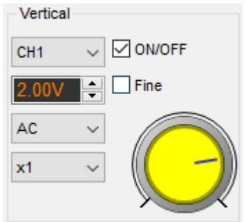
**Note:** The attenuation factor changes the vertical scale of the oscilloscope so that the measurement results reflect the actual voltage levels at the probe tip.
