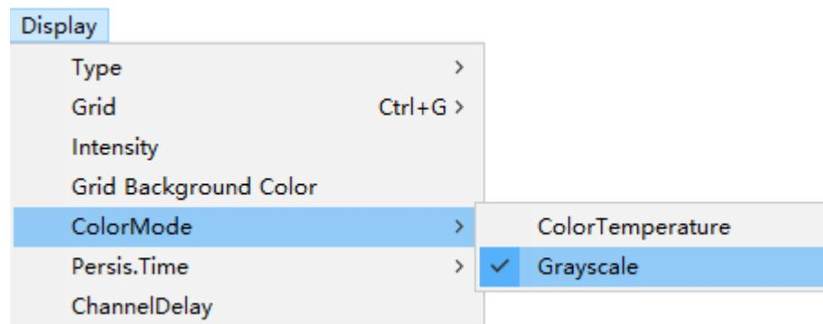
There are two kinds of grayscale display mode, When choosing a DPO mode for level 256 grayscale display and the max waveform capture rate to 60,000 wfm/s, but if the Acquire is on the FastAcq model, so the oscilloscope is only with 1-level intensity grading display function and the max waveform capture rate to 400,000wfm/s.
