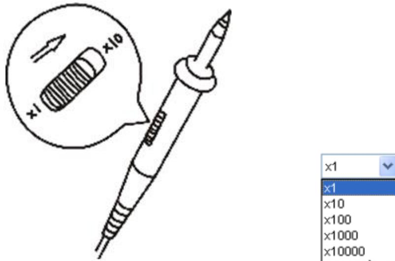
3. Attach the tip of probe and ground clip to the Connector of Probe compensator. Click the
