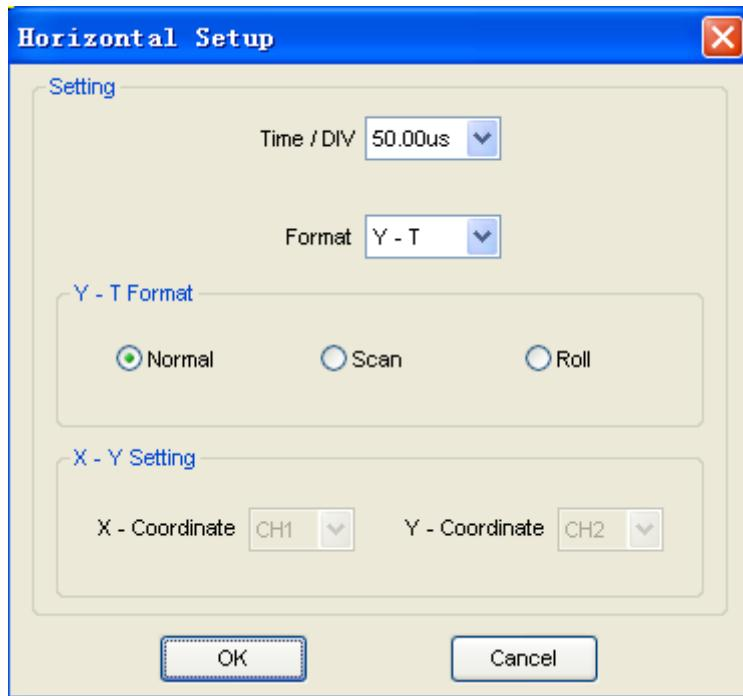
1. **Time/DIV:** leads the setting of the time base parameters
