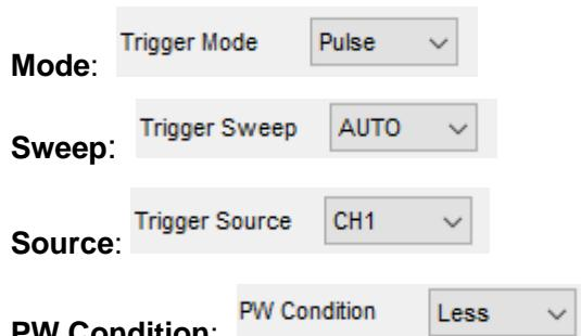
**Pulse Width:** The Pulse Width adjust range is 10ns~10s. When the condition is met, it will trigger and acquire the waveform.
