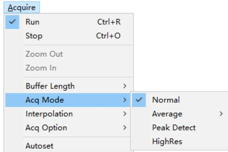
**Normal:** In this acquisition mode, the oscilloscope samples the signal in evenly spaced intervals to construct the waveform.
