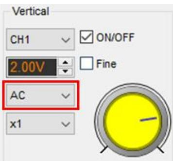
You can set the coupling to **DC**, **AC** or **GND**. If you set the coupling to **DC**, it blocks the **AC** component of the input signal.
