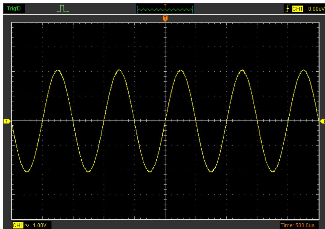
If the **Dots** type mode is selected, the waveform will be displayed as following figure.
