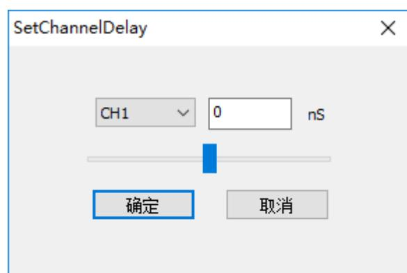
When using the oscilloscope for actual measurement, the transmission delay of the probe cable may cause relatively larger error (zero offset). Zero offset is defined as the offset of the crossing point of the waveform and threshold level line relative to the trigger position. You can set a delay time to calibrate the zero offset of the digital channels. The range is from
