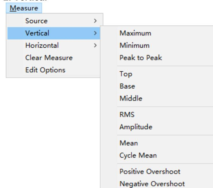
**Maximum:** Voltage of the absolute maximum level, Measured over the entire waveform
