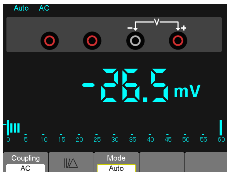
Figure 7-7 AC voltage Measurement
